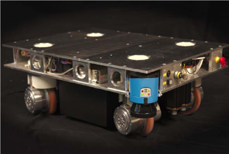
Figure 2. The rob@work mobile platform is used as the platform to realize the envisioned robot-based training system
