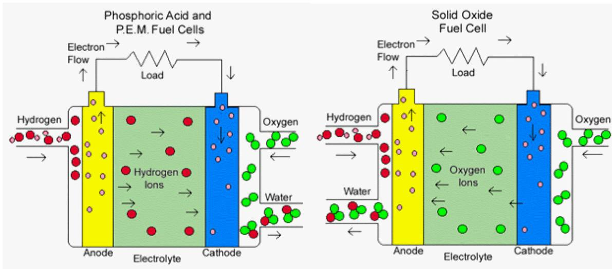
The efficiency of fuel cells is little dependent on scale and fuel cells are used in applications from mW to MW scales – in vehicles and trains, auxiliary power supply units, combined heat and power units, etc. High temperature fuel cells may be combined with gas turbines (hybrid systems) to achieve a higher overall electricity efficiency.
