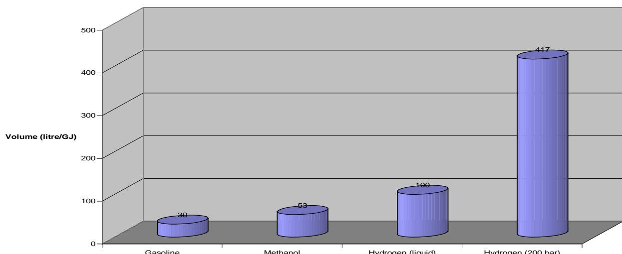
The illustration compares the volume (in litres) needed by different energy carriers for holding the same amount of energy (1 GJ).
