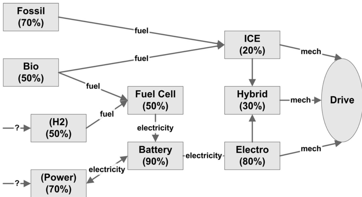
The above figure illustrates typical energy efficiencies (in %) at the various steps in different energy chains from the energy sources to the final energy service, here the drive of a mobile application - from well to wheel. The total efficiency varies from 10% (Bio- - Internal Combustion Engine (ICE) - Drive) to 50% (Power - Battery - Electro - Drive).
