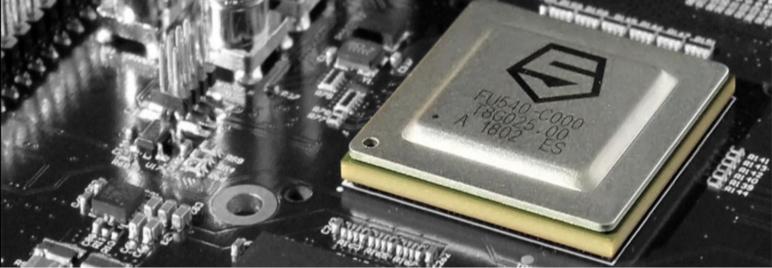
Fig. 9: HiFive Unleashed board with the 64bit RISC-V Freedom U540, which is a Linux-capable, multi-core processor up to 1.5 GHz. (Source: https://www.sifive.com/products/hifive-unleashed/ )
