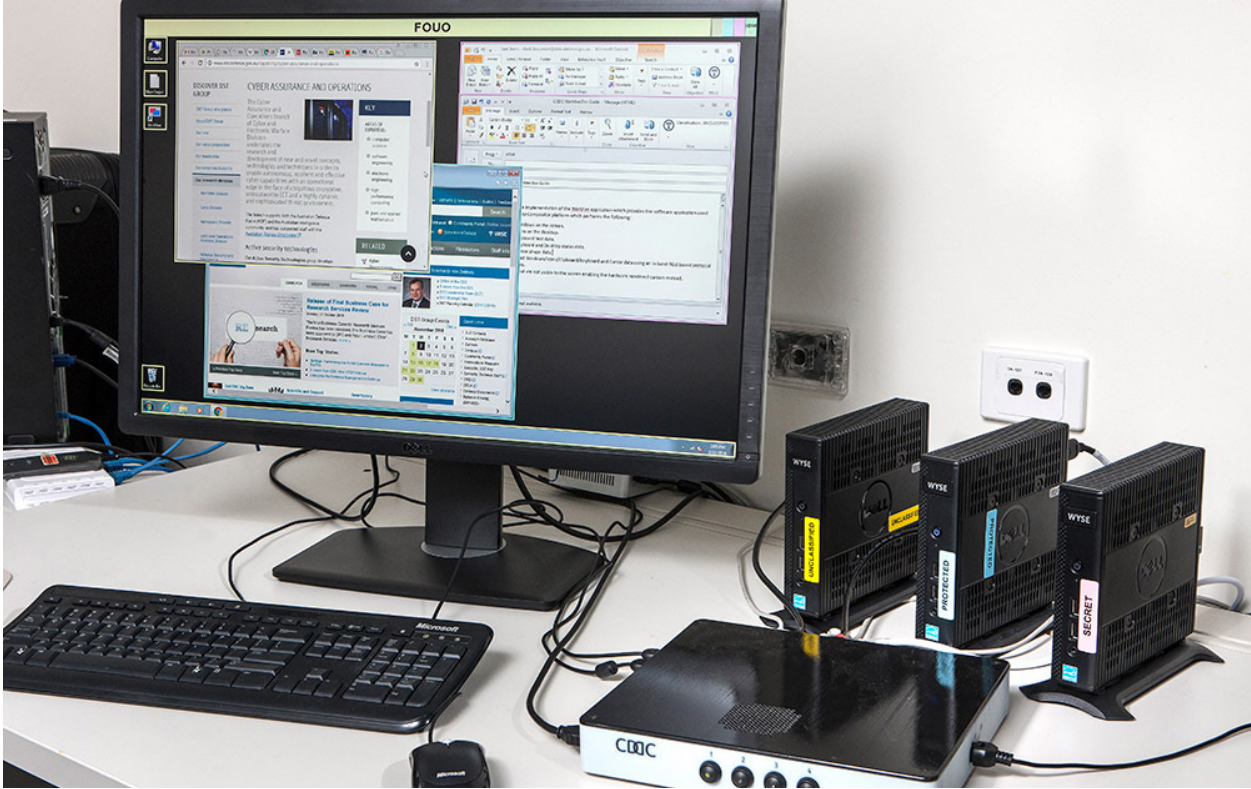
Fig. 12: Cross Domain Desktop Compositor. In this example designed for use in the armed forces, unclassified, protected and secret information is kept separate while managed from the same user interface. This approach could be used to handle legacy systems while migrating towards a new, more secure one ( https://research.csiro.au/atsblog/cddc-wins-iawards/ ).
