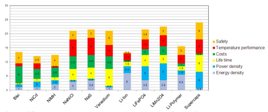
Comparison of different battery systems regarding technological aspects, without consideration of a specific application field and weighting system. (Weil, M.; Decker, M.; Fleischer, M.; Frankenberg, A. 2011)
