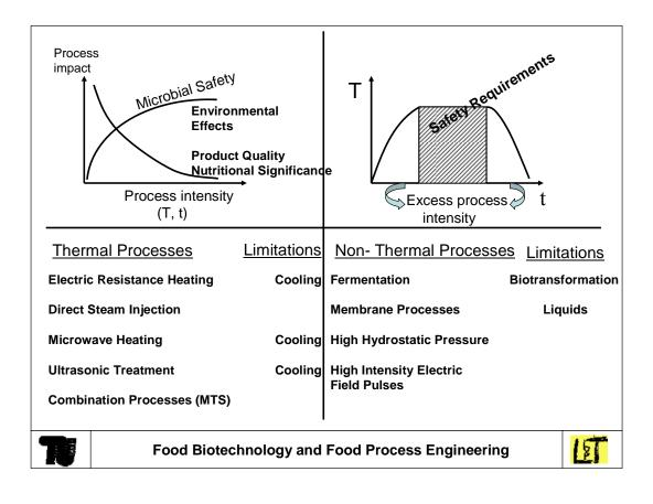
Fig 2: Principle advantages and process application of key advanced technologies.
